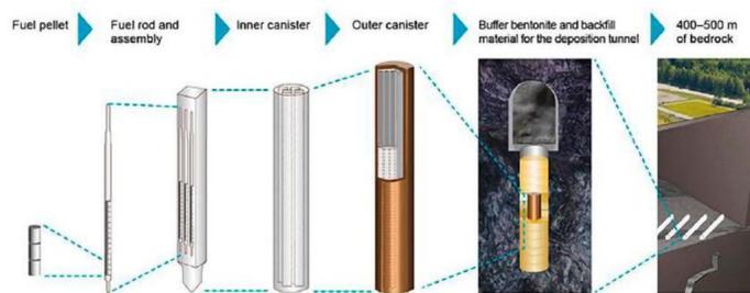
Multibarrier principle in the KBS-3V repository concept. Illustration courtesy of Posiva Oy.
